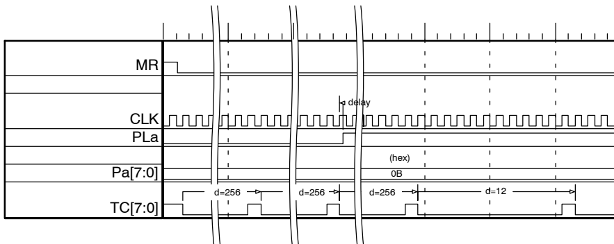
Figure 14. Timing Diagram for PLa / PLb Inputs (After Critical Rising Edge of CLK) (SEL is Low)
